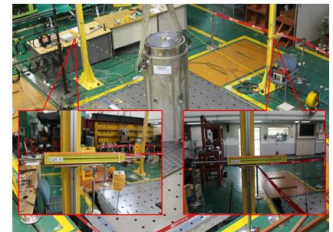
LVDT 변위계: SDF-300D : 2ea
